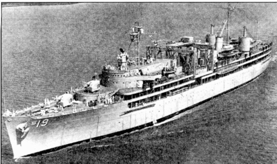
Originally built as a 10,100-ton Fulton-class submarine tender, USS Proteus (AS-19) was launched late in 1940 at Mare Island. After extensive wartime service she was lengthened and converted to support Polaris missile submarines in 1959/1960. Later, she received a FRAM II refit to accommodate nuclear submarines. This early 1970s photo show Proteus still armed with her wartime battery of four 5-in/38s in single mounts. Her guns were removed during a 1975 refit.
